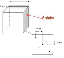
The aim of the test is to compare the real distances between markers to that measured by the audited center.
