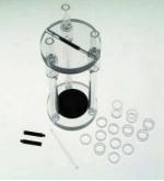
Up to 11 TLDs are irradiated in photon beams and up to 5 TLDs in electron beams.
