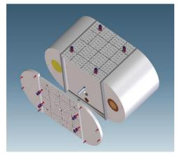
Up to five dosimeters are irradiated separately, in the plastic phantom that contains inhomogeneities mimicking bone tissue, lung tissue and air.
