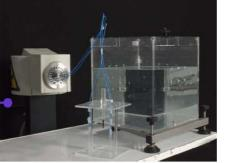
Dose measurements are performed in water, using an appropriate holder that allows positioning applicators around the TLD in a triangular configuration.
