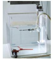
TLDs are placed in the water using special designed holder for each type of beam.
